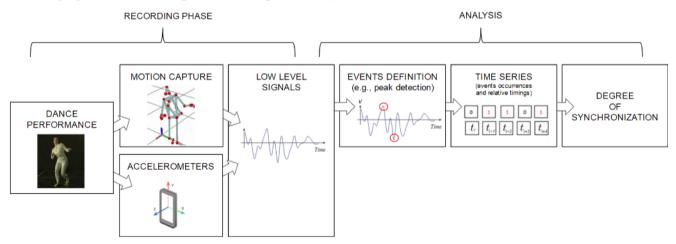
The dancer's movement is captured by either a set of markers of a motion capture system or a set of accelerometers. Signals representing the user's limbs velocities are computed. By applying the peak detection algorithm described in Section 2.2.1.1 we obtain one timeseries per limb, containing zeros when no peak is detected and ones when a peak is detected. We compute the degree of synchronization between pairs of timeseries.
